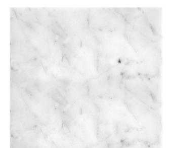
Variation in color, shade, finish, hardness, strength and slip resistance is inherent in Natural stone products. White marbles contain naturally occurring deposits of iron which may lead to discoloration of marble and turning it yellow-rust or grey if used in wet areas. This a natural characteristics of the stone and that is why it cannot be considered as a defect
