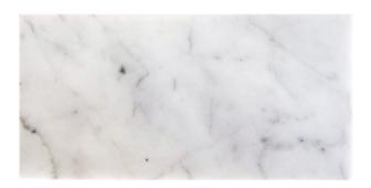
Variation in color, shade, finish, hardness, strength and slip resistance is inherent in Natural stone products. White marbles contain naturally occurring deposits of iron which may lead to discoloration of marble and turning it yellow-rust or grey if used in wet areas. This a natural characteristics of the stone and that is why it cannot be considered as a defect
