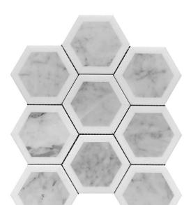
Variation in color, shade, finish, hardness, strength and slip resistance is inherent in Natural stone products. White marbles contain naturally occurring deposits of iron which may lead to discoloration of marble and turning it yellow-rust or grey if used in wet areas. This a natural characteristics of the stone and that is why it cannot be considered as a defect
